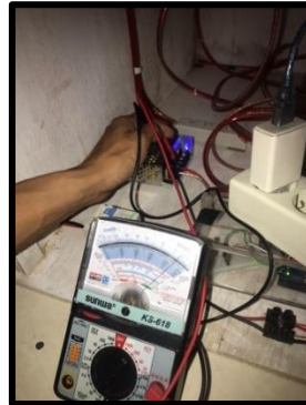
Gambar 6. Pengujian Power Supply
